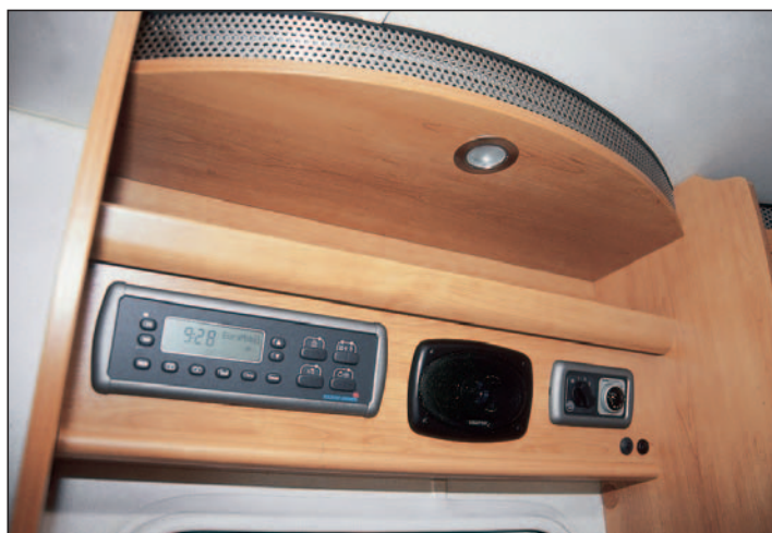
Above the caravan door are the control panel, a radio speaker, and control for the water and blown-air heating. The metal strip adjoining the ceiling is an outlet vent for the ISO cooling system. There are similar outlets strategically placed throughout the 'van.
