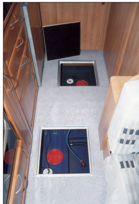
Fresh and waste water tanks are enclosed within the double floor cavity. The small unit to the right of shot, behind the seatback, contains the waste bin.
