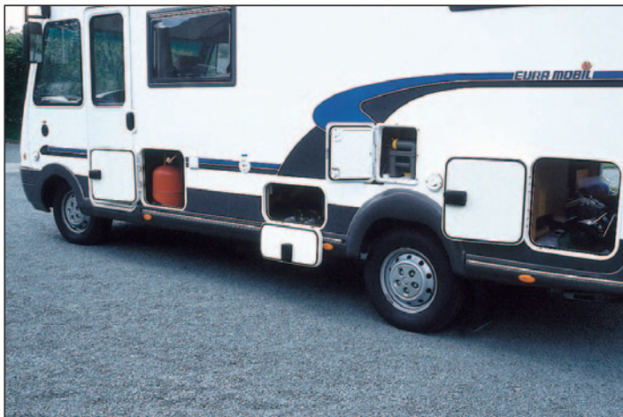
All utilities are accessed on the nearside, including a small door for the rear underbed storage area.
